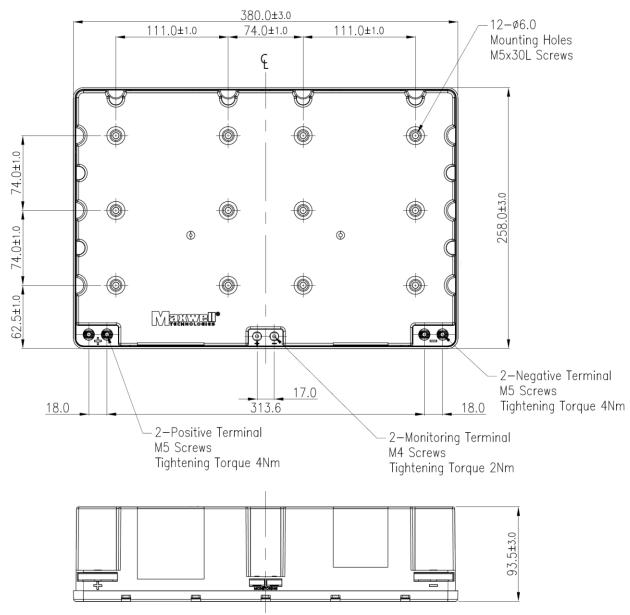
Figure 2: BMOD0010 Mounting Hole Locations
