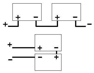
**Figure 3: Possible Series Connection Arrangements**
