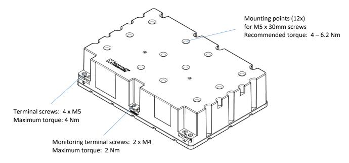
Figure 1: BMOD0010 Mechanical Configuration
