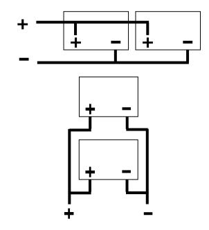
**Figure 4: Possible Parallel Connection Arrangements**
